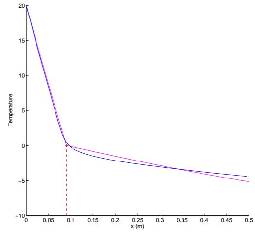
Figure 2: Temperature profile at  $t = 50 h$ .  $\Delta T = 1^\circ C$ . Analytical (red) and numerical (blue) solutions.
