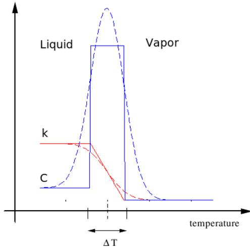
Figure 1: Estimation of thermophysical properties in phase change problems.
